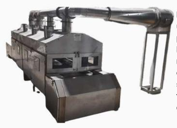
Novel Continuous Refractance Window Drying uses low temp. and short-time continuous process to dry delicate, heat-sensitive products. Drying takes place at atmospheric pressure to retain product color, Flavor, aroma and nutritional content. Product quality is comparable to and, in some instances, better than that achieved by freeze-drying, spray drying, drum drying. This is done at signicantly less capital and energy cost.
